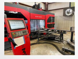
The Akyapak 3 ADM 1200 CNC Beam Line can perform complex operations in an efficient process with the multitasking capability of cutting, drilling, marking, milling, tapping, and countersinking. It features 22Kw spindle motors, 500 mm sub-axis and three drill spindles each with a 6-station automatic tool changer. It also automatically feeds the material with accurate material measurement with full automated material transfer from start to finish.
